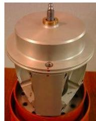
If blade angles are not identical – then you have to correct the tiny little play between the rod end and the bolt M6 that causes this difference.
