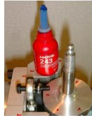
Insert hexagonal bolt M6 with Loctite 243 (blue) and place the washer between the rod end and the main axle.
