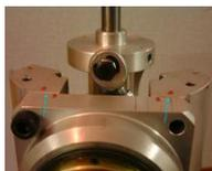
If necessary center the play between the four bolts M8 and the holes in the aluminum root bracket in order to allow contact of the front cap only to the hub, not to the brackets.
